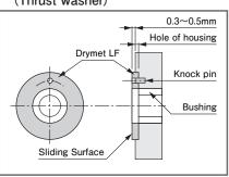
**%** Sliding surface consists of a plastic layer.
